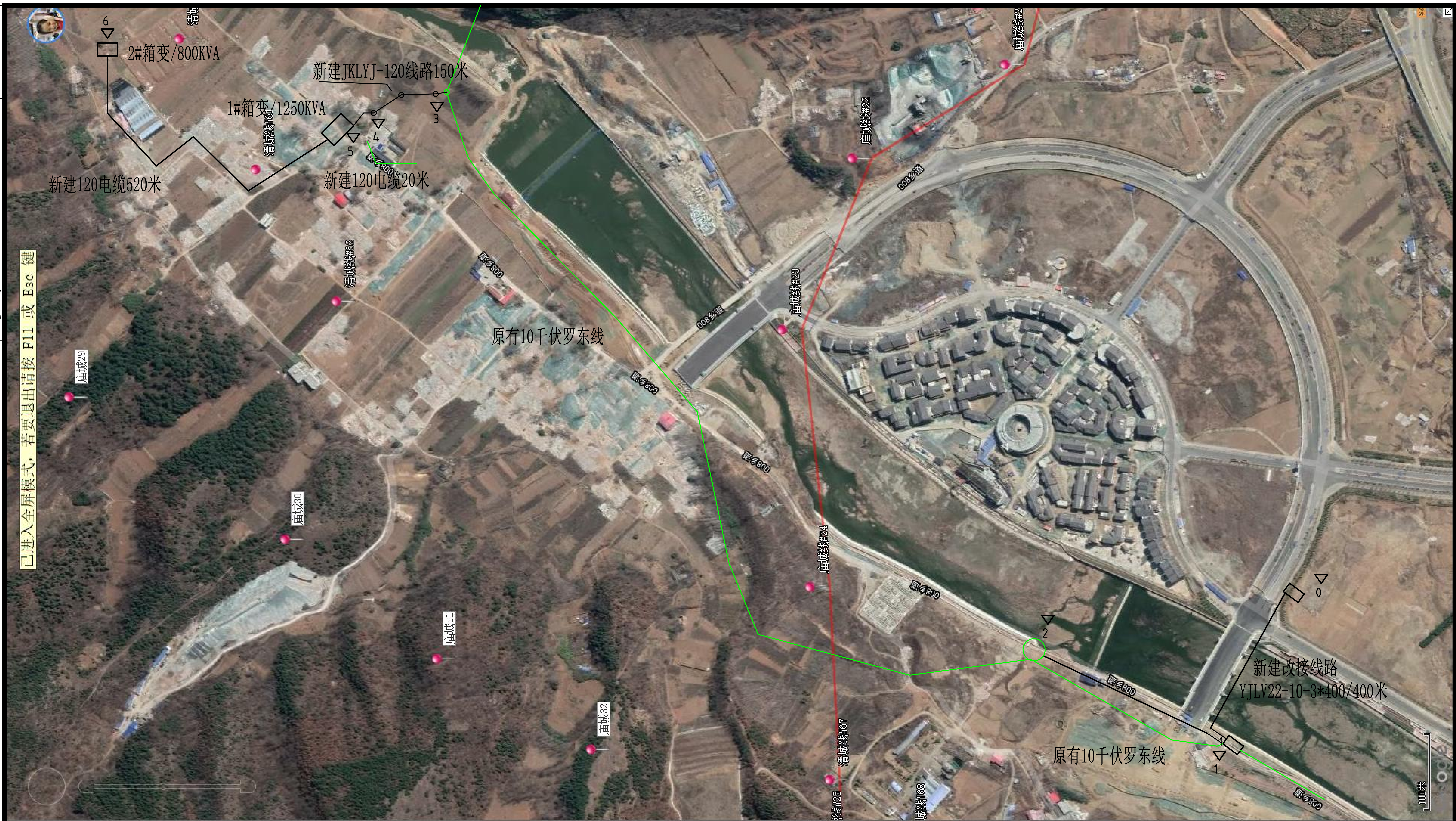
电缆敷设区段表 (3×400/400m+架空150米+3×120/540m)
